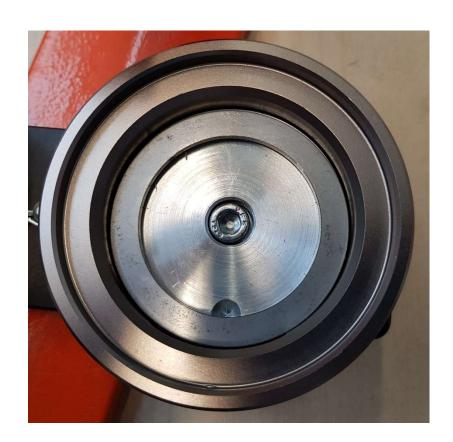
Make sure metal ring is in the bottom of die B
