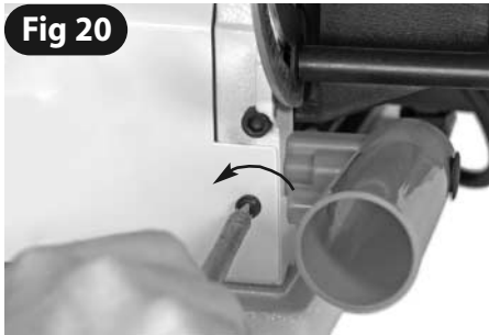
Fig 20 To gain access to the drive bearings, remove the side panel by undoing the Philips screw, counter-clockwise.
