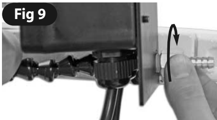
Screw the 1/4" BSP fitting back on the air tube assembly using a 17mm spanner
