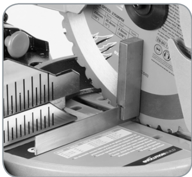
Fig. 12 View of Engineers Square in position
