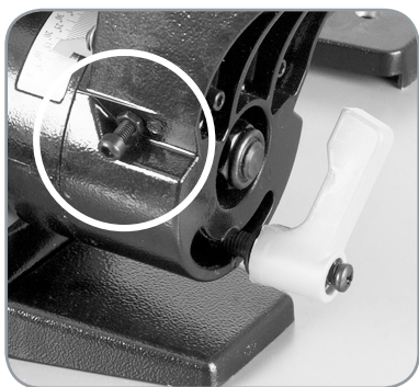
Fig. 13 Close up view of Adjustment screw and locknut
